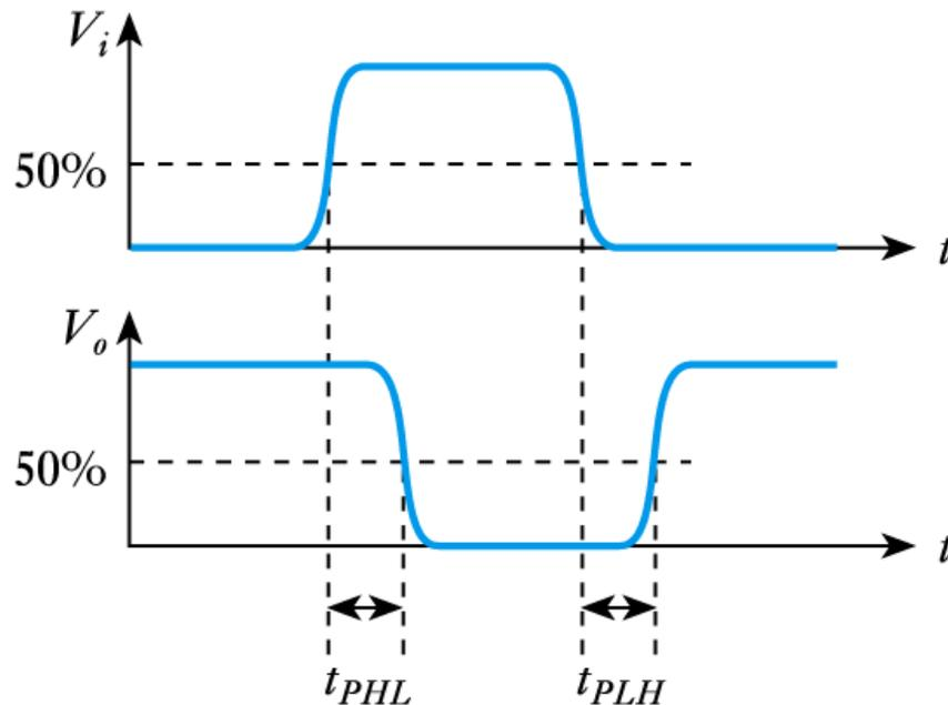
$$t_{PD} = \frac{1}{2}(t_{PHL} + t_{PLH})$$
