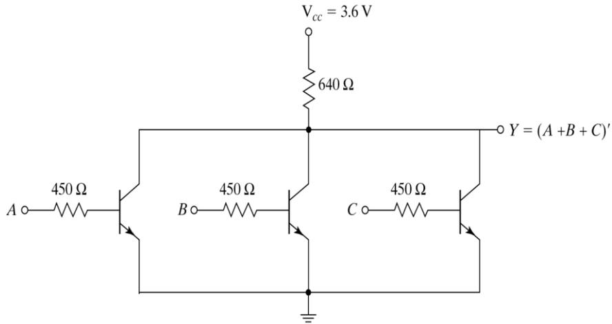
Fig. 10-8 RTL Basic NOR Gate
