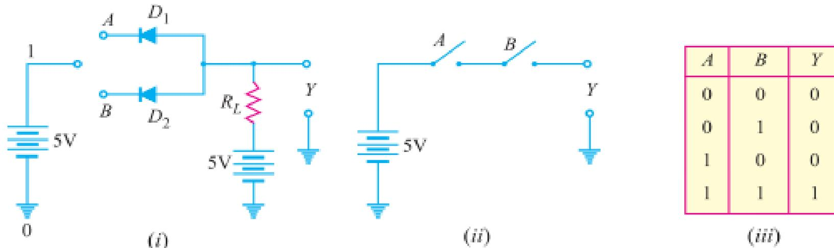
**(i)** When both  $A$  and  $B$  are connected to ground, both the diodes ( $D_1$  and  $D_2$ ) are forward biased and hence they conduct current. Consequently, the two diodes are grounded and output voltage is zero. In terms of binary, when  $A = 0$  and  $B = 0$ , then  $Y = 0$  as shown in truth table in Fig. 26.8 (iii).
