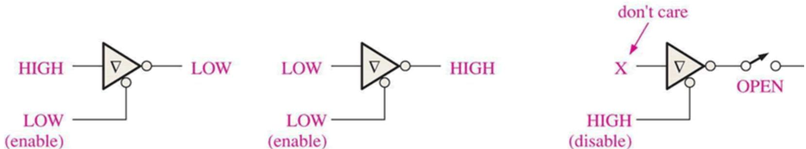
(a) Enabled for normal logic operation
