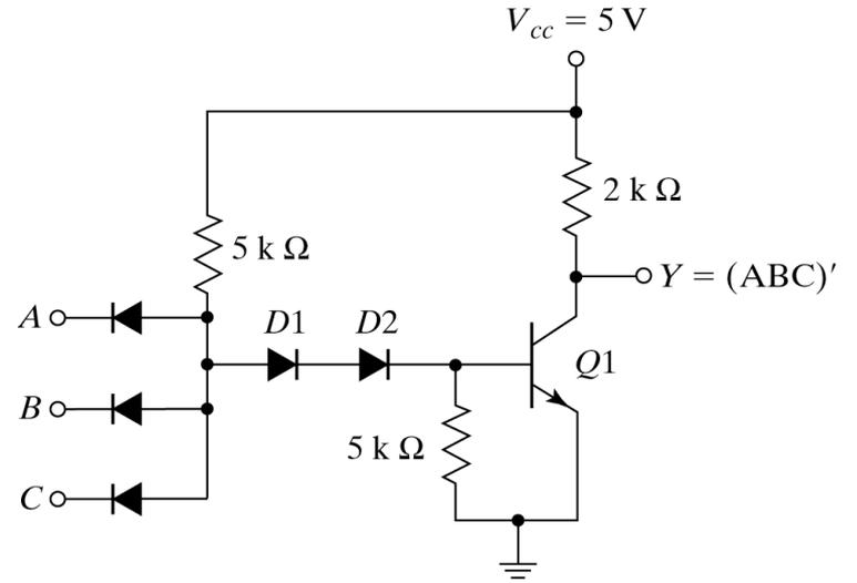
Fig. 10-9 DTL Basic NAND Gate
